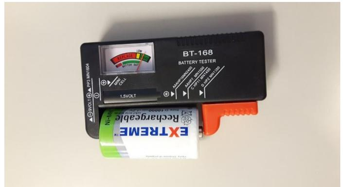
7. **How to test the batteries:** simply push the red slider as far to the right as it will go and insert the battery into the space (with positive charge on the right, next to the slider). Read the display to check that it says 'good'.
