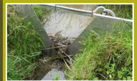
One of the more unusual challenges of working within a beaver enclosure is that water trickling through v-notch weirs triggers this instinctive behaviour by the beavers.
