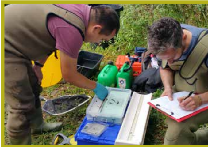
Fish were caught by electrofishing above and below a beaver dam, and recorded in detail.
